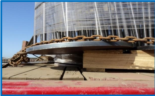
This load is secured with chains, however only 50% of the load is on the pallet.
