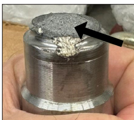
Final fracture of hook shank
