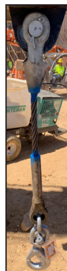
Swivel Shur-Loc (no rotation under load)
